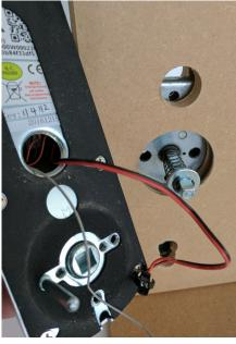
3. Insert the latch support pin on the inside of the front plate in either outer hole.
